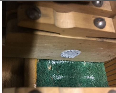
RMT 79-6, piano. Lead weight in contact with wooden keys.
