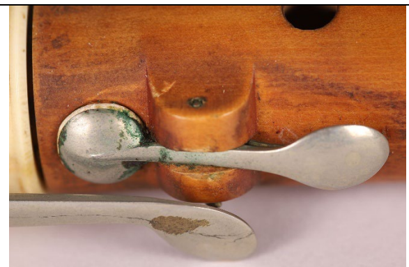
RMT 88-8, flute. New silver in contact with wood.
