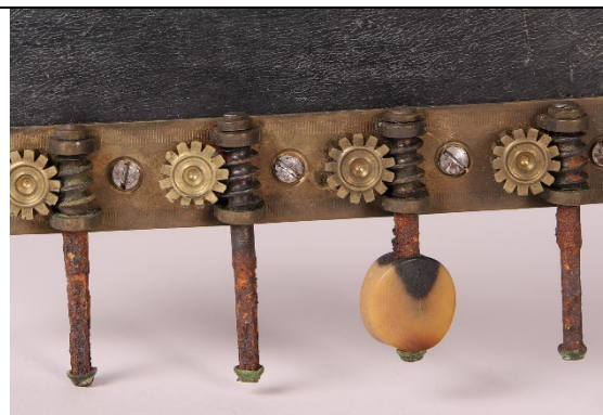
RMT 547, mandolin. Steel core of screw in contact with plastic.
